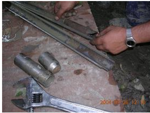
Figure 4: Soil sampling using SPT
