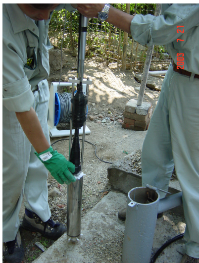
Fig 11: Seismic instrumentation of borehole
