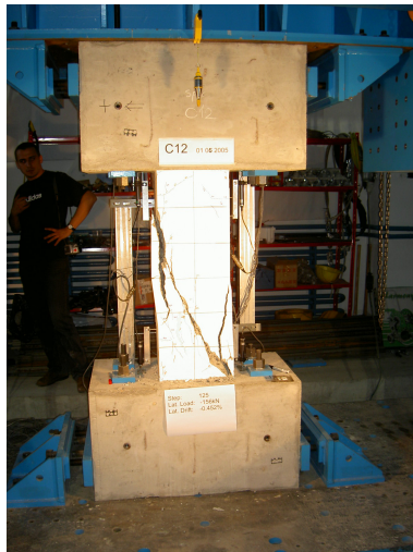
Figure 7: Test on RC columns (original specimen, retrofitted specimen with steel plate and with CF sheet)
