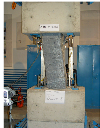
Figure 7: Test on RC columns (original specimen, retrofitted specimen with steel plate and with CF sheet)
