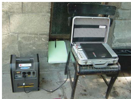
Fig. 15 Data acquisition system for PS logging
