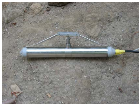
Fig. 14 Borehole sensor for PS logging
