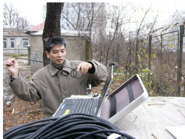
Microtremor data acquisition by Dr. Koyama at seismic stations sites
