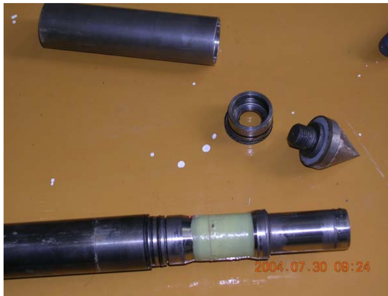
Electric cone C10CFIP
