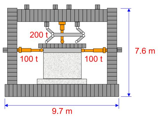
Reaction frame to be installed at UTCB
